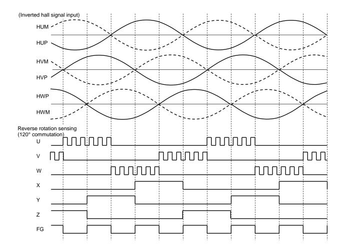
\*: When CW/CCW = Low, inverted Hall signals put the TB6584FNG in 120 commutation mode with a lead angle of 0° (reverse rotation).
