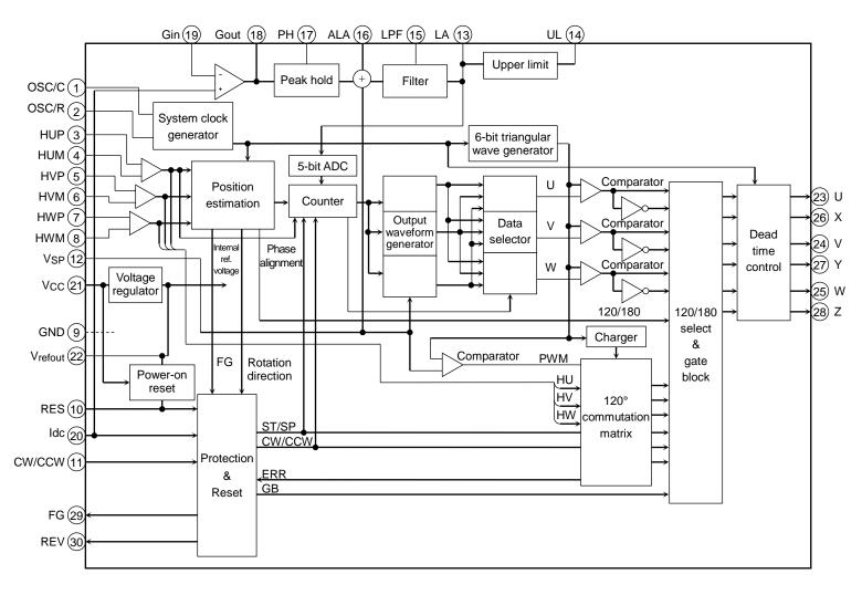
In the above block diagram, part of the functional blocks or constants may be omitted or simplified for explanatory purposes.
