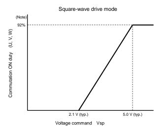
Note: The conduction time is reduced by the dead period. (carrier cycle  $\times$  92% – T<sub>d</sub>  $\times$  2)
