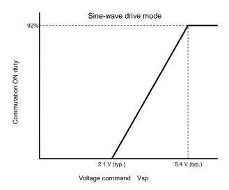
The position signals from Hall sensors are modulated, and the modulated signals are then compared against a triangular waveform to generate a sinusoidal PWM waveform.
